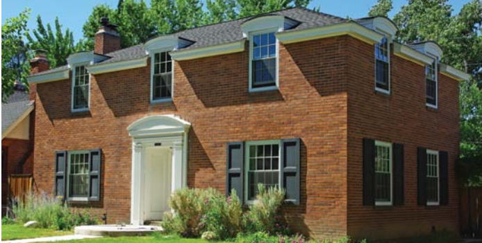
This Colonial Revival style residence on Manor Drive features interesting through-the-cornice dormers with segmental heads.
